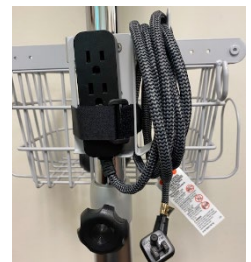
2.f Attach the Power Cord Extension to the Cord Cleat and organize the cord.
