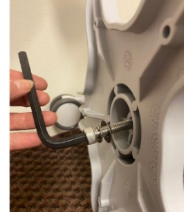
1.c Lay assembly on its side to access the base bottom. Grip the post to prevent rotation. Secure the post to the base using the Hex Wrench. Return stand to upright position.
