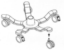
1.a Install the casters onto the base.
