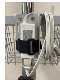
2.f Attach the Tablet's Power Cord to the Cord Cleat and organize the cord.
