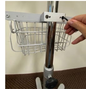
2.c Slide the Basket onto the upper post opposite the Adjustment Knob. Position the Basket approx. midway down the post and tighten the bracket evenly.
